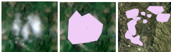
Figure 4. Clouds and shadows present in maps from each date were masked using polygons and aggregated into one shape file
