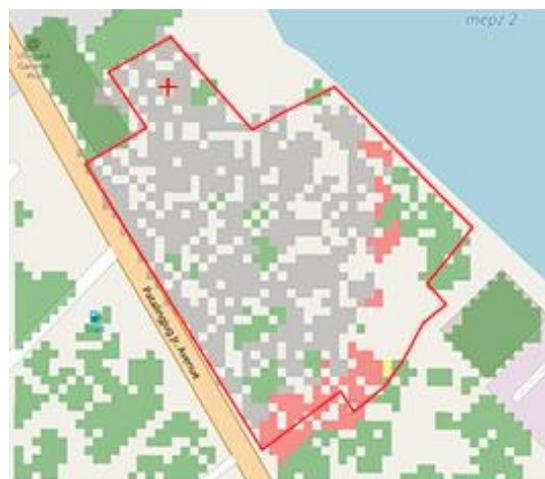
Figure 11: Completed fire spread simulation (actual extent outlined in red, fire origin marked by '+')
