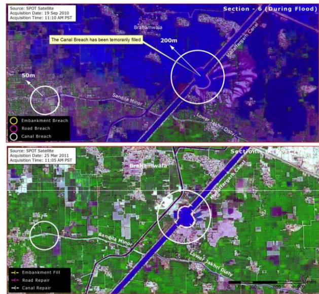
Figure 7. Filling of Muzaffargarh Canal Breach, Punjab
